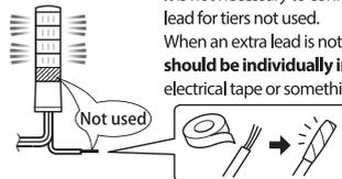
It is not necessary to connect to an external lead for tiers not used. When an extra lead is not connected, it **should be individually insulated** with electrical tape or something similar.
