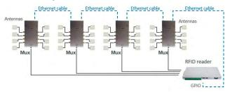
AdvanMux-8 can be controlled both by standard +5 V and open collector digital outputs.
