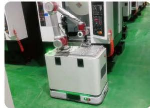
Composite robot CNC loading and unloading
