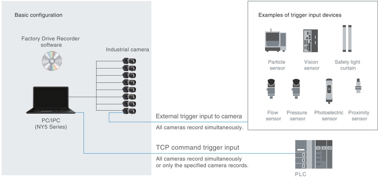
Note: Up to eight cameras can simultaneously record. A hub is required to connect cameras depending on the PC specifications and the number of connected cameras.
