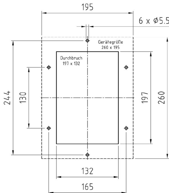
**FL-208-AC (Peltier-Gehäusekühler) | Art. Nr. 2116****5 ZERTIFIKATE UND HINWEISE****ZERTIFIKATE**
