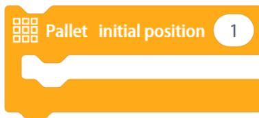
(1) Meaning: Set the pallet type, point number and gap number to make the robot execute the pallet program.
