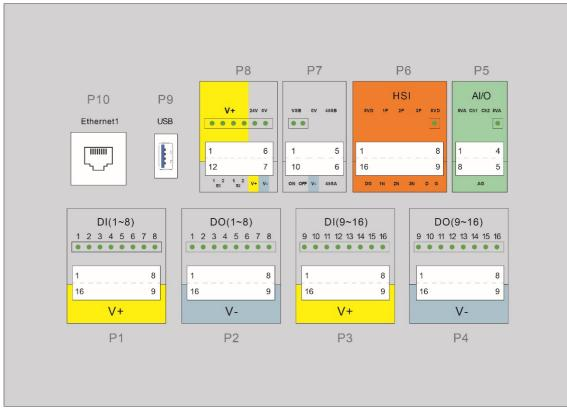
Figure 4-1 Front panel interface of the electrical cabinet
