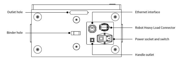
Figure 4-15 Electrical cabinet bottom panel interface
