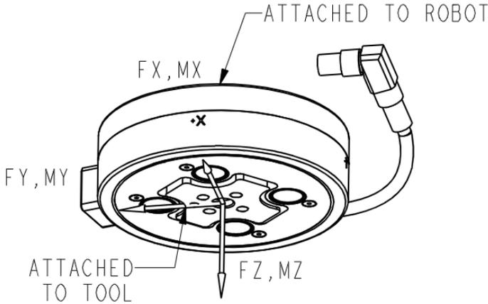
Figure 2-25 Definition of the Sensor Coordinate System
