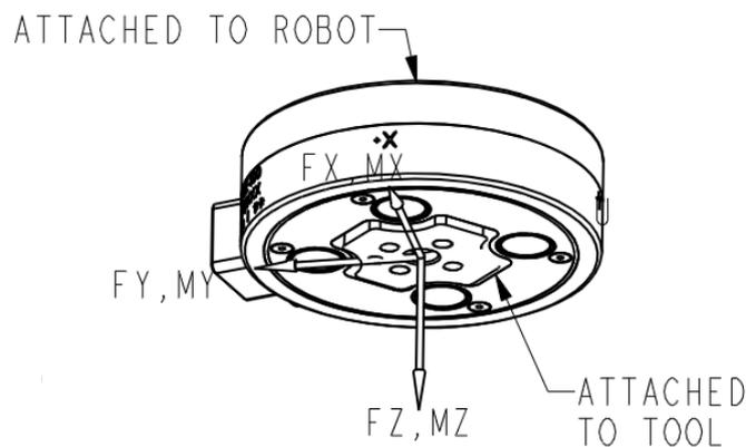
Figure 2-12 Definition of the Sensor Coordinate System
