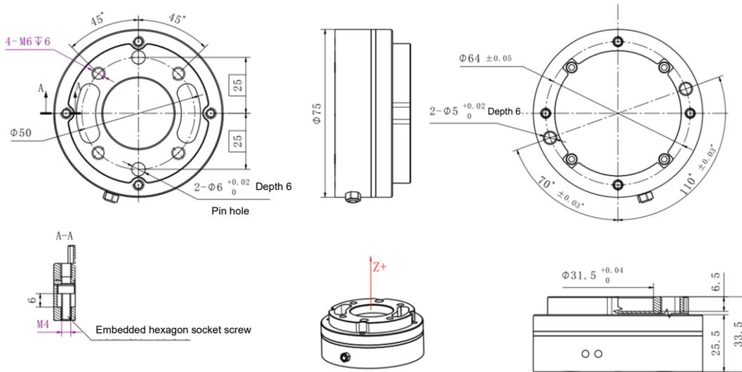
Figure 2-18 Sensor Dimensions
