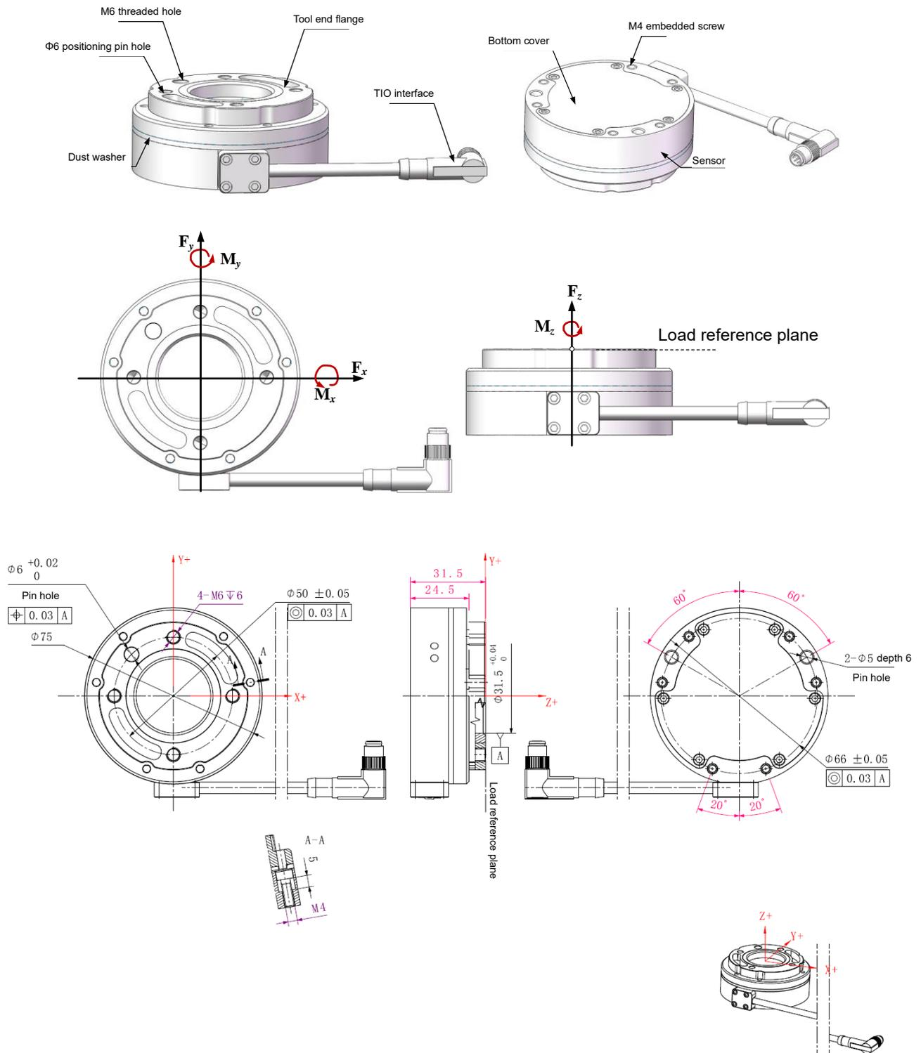
Figure 2-26 Appearance and Dimensions of the Sensor
