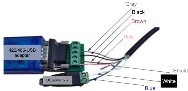
Figure 2-11 Wiring of the 422/485-USB Adapter and Power Plug
