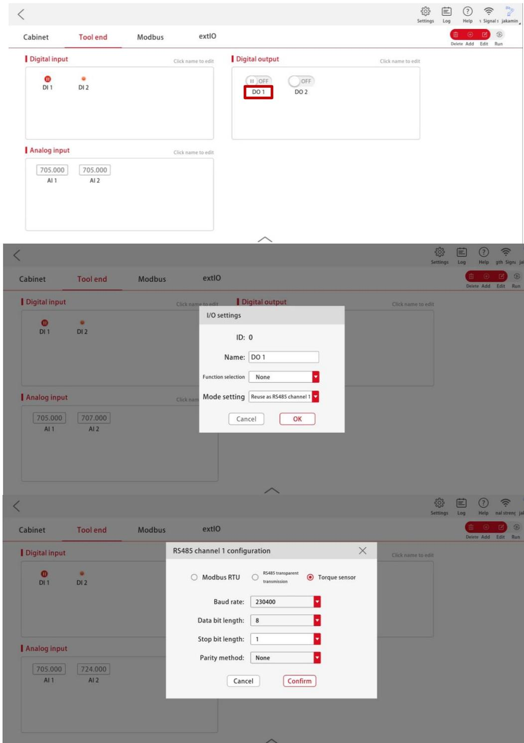
Figure 3-6 RS485 Channel Configuration Interface
