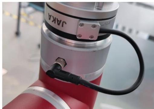
Figure 2-30 Cable Connection
