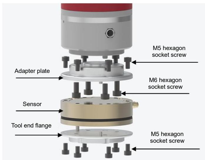
Figure 2-2 Sensor Installation
