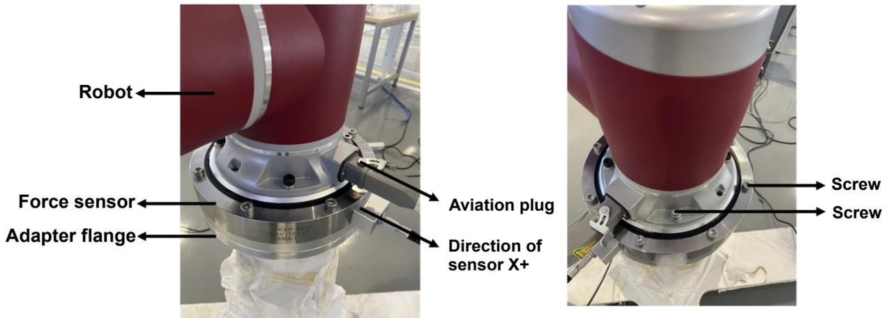
Figure 2-42 Installation of Type IV Sensor
