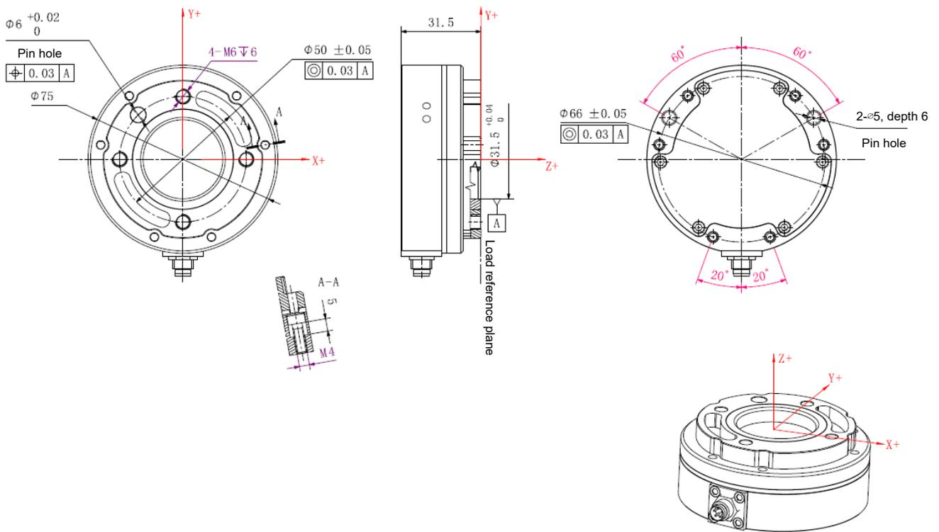
Figure 2-6 Sensor Dimensions
