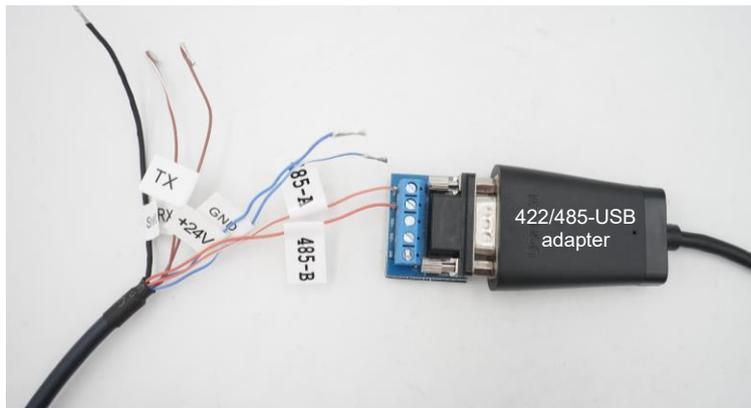
Figure 2-40 Wiring of the 422/485-USB Adapter and Power Plug
