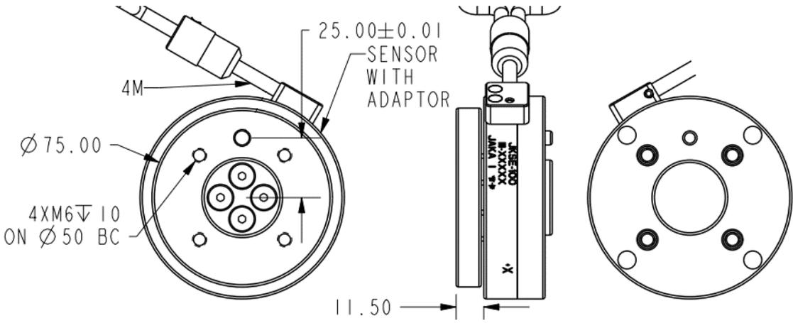
Figure 2-38 Installation and Dimensions of the Sensor
