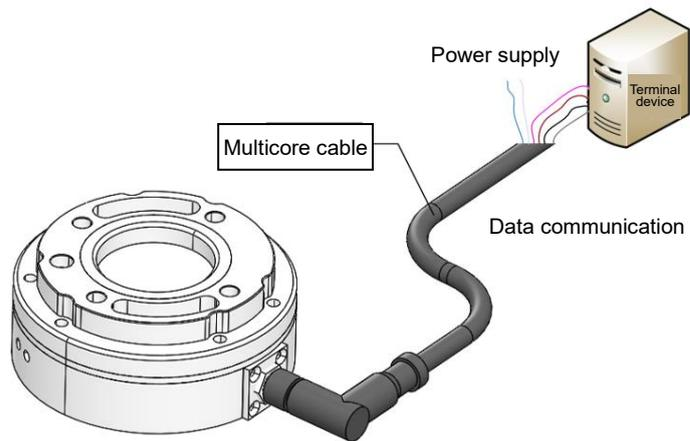
Figure 2-5 Electrical Connection of the Sensor
