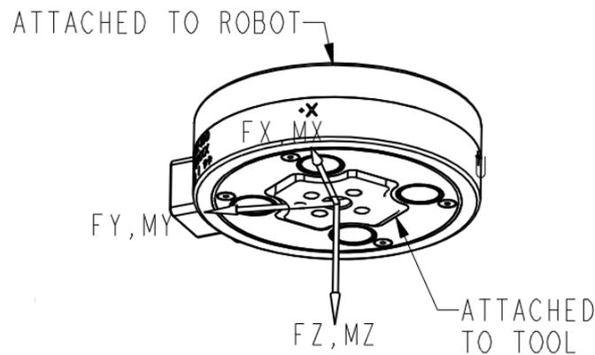
Figure 2-37 Definition of the Sensor Coordinate System
