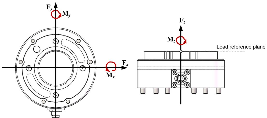
Figure 2-4 Definition of the Sensor Coordinate System
