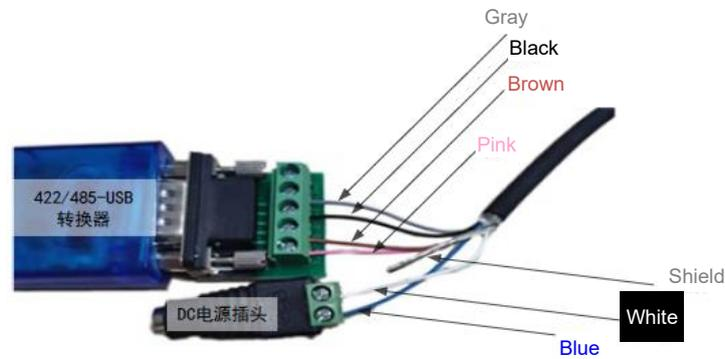
Figure 2-23 Wiring of the 422/485-USB Adapter and Power Plug
