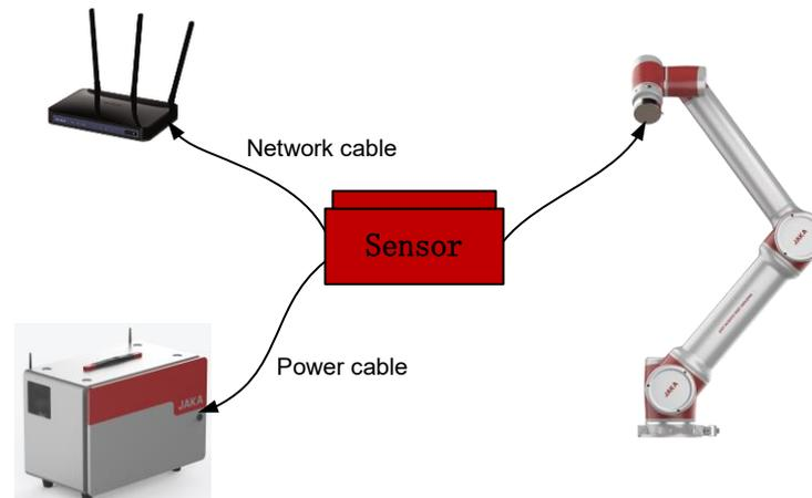
Figure 3-1 Se System (Network Port Type)
