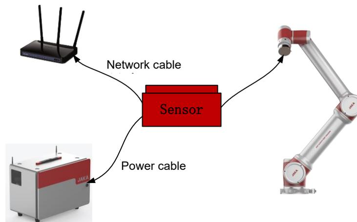
Figure 3-16 Se System (Network Port Type)
