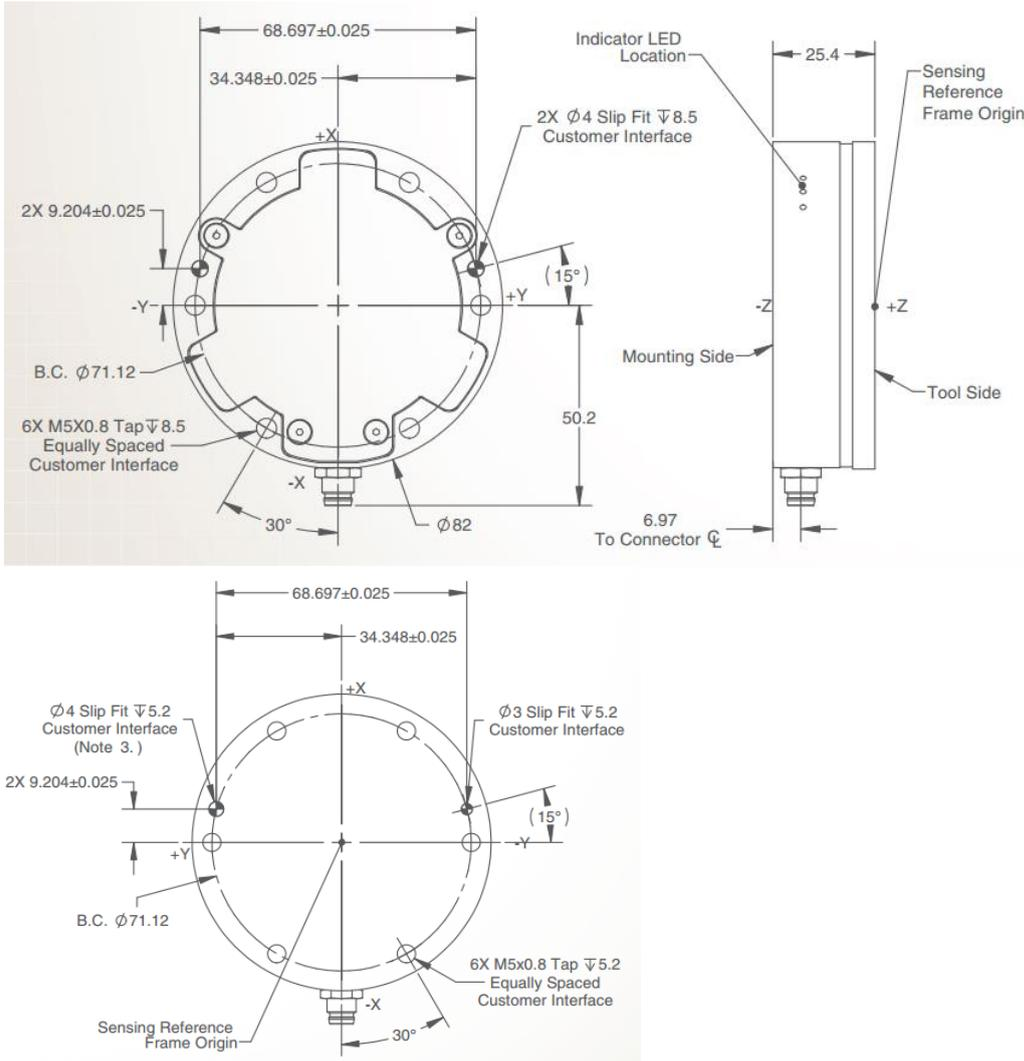
Figure 2-1 Dimensions of the Sensor
