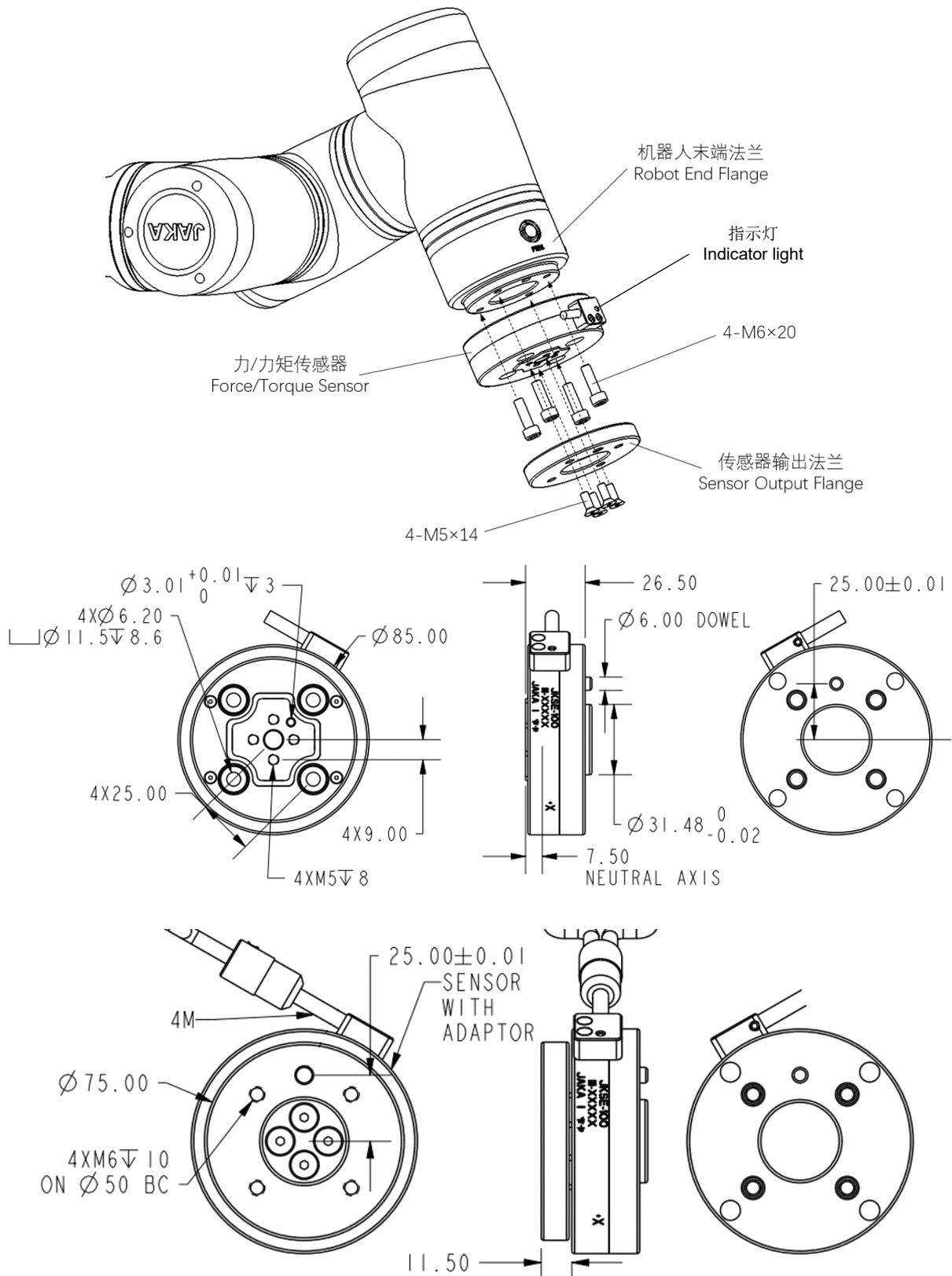
Figure 2-13 Installation and Dimensions of the F/T Sensor
