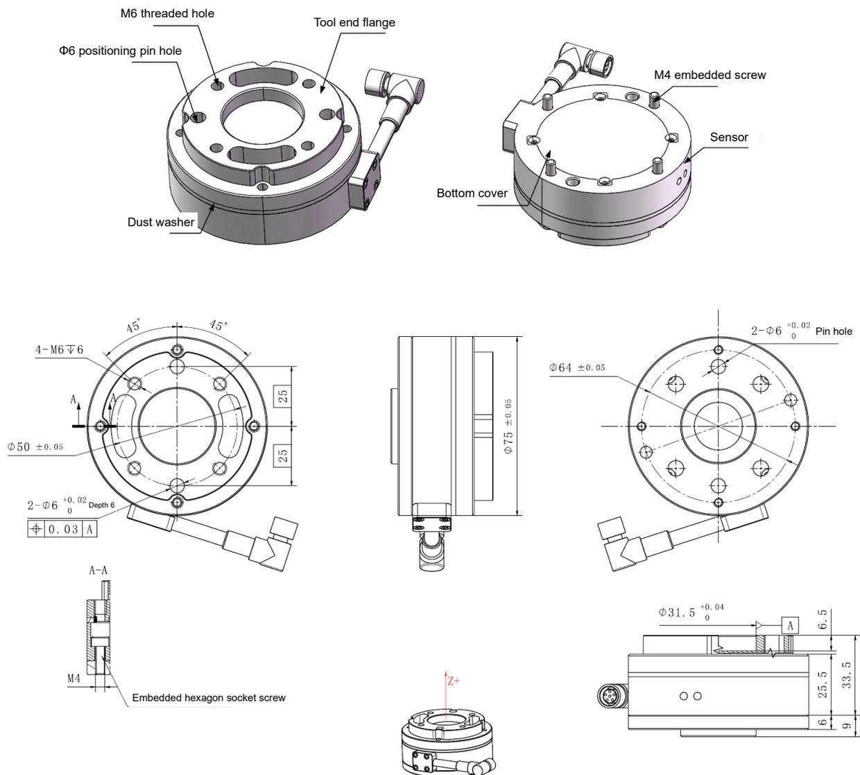
Figure 2-31 Sensor Dimensions
