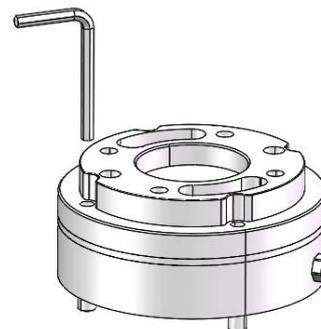
Figure 2-20 Loosen Embedded Screws Using a 3 mm Allen Key
