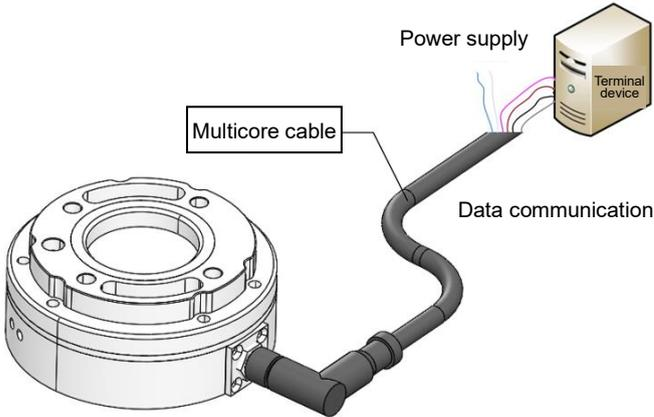
Figure 2-17 Electrical Connection of the Sensor
