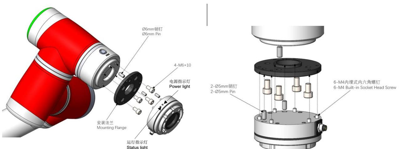
Figure 2-9 Installation of the Sensor to the Robot
