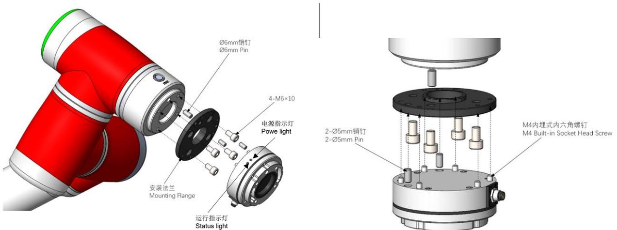
Figure 2-34 Installation of the Sensor to the Robot
