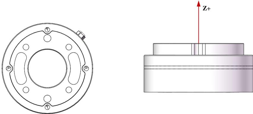
Figure 2-16 Definition of the Sensor Coordinate System
