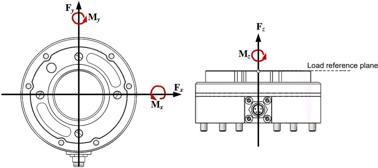
Figure 2-24 Definition of the Sensor Coordinate System
