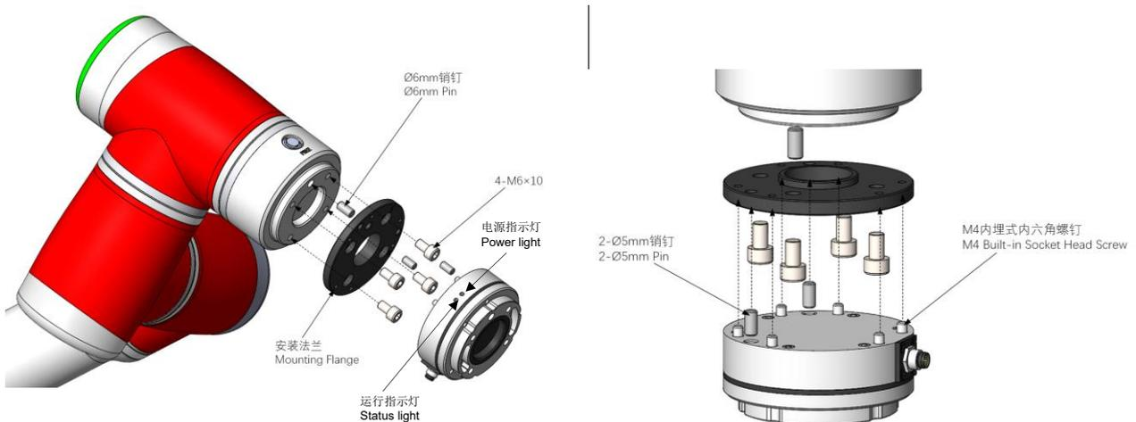
Figure 2-21 Installation of the Sensor to the Robot
