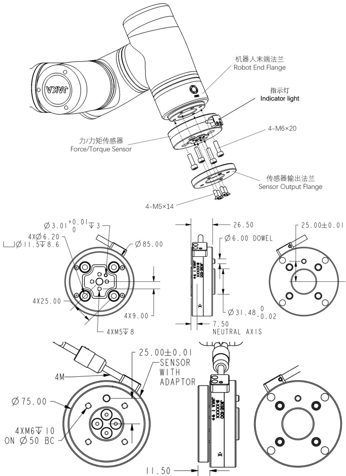
Figure 2-36 Installation and Dimensions of the Force Sensor
