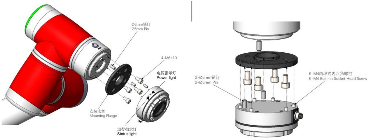
Figure 2-29 Installation of the Sensor to the Robot
